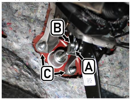
2. From the engine bay, disconnect the rubber Reservoir Hose at the inlet port and remove the Clutch Master Cylinder Assembly.
